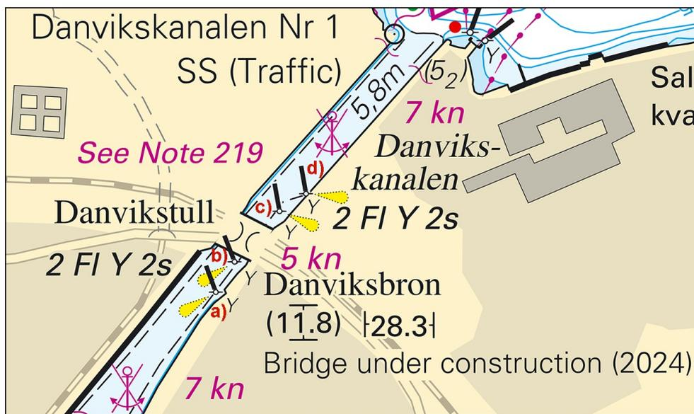
New special purpose light spar buoys in the canal 'Danvikskanalen'
