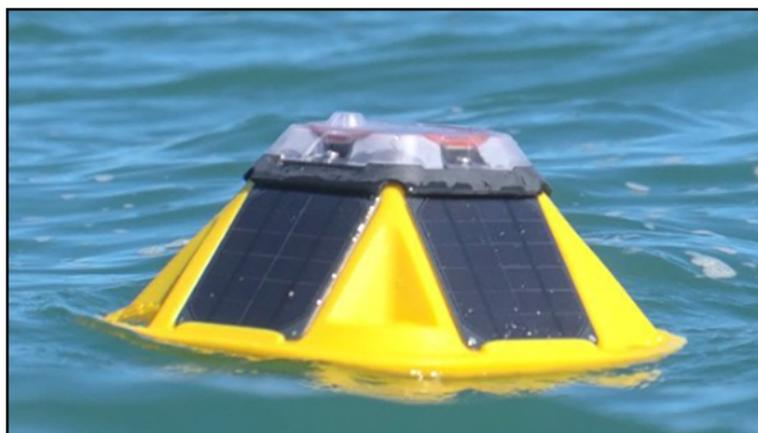
Wave sensor buoy
